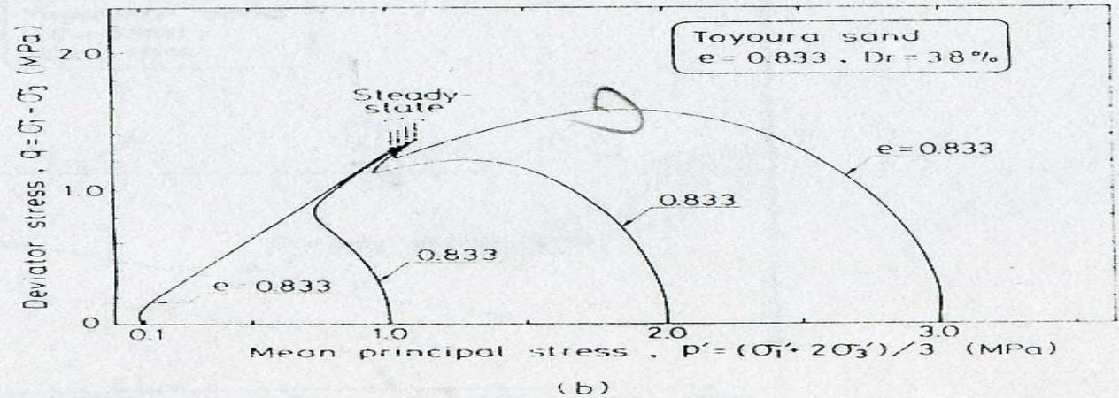
Fig. 27. Undrained behaviour of medium loose sample of Toyoura sand.
