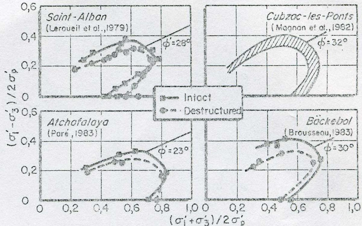
Figure 2. Limit state curves of intact and destructured natural clays.
