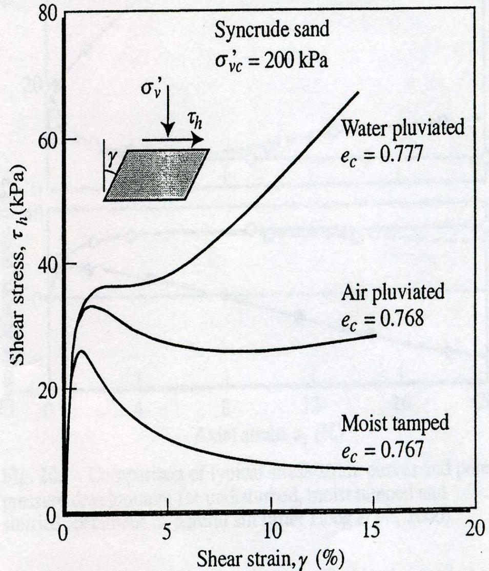
Fig. 19. - Effect of specimen reconstitution method on undrained simple shear response (after Vaid *et al.*, 1995)
