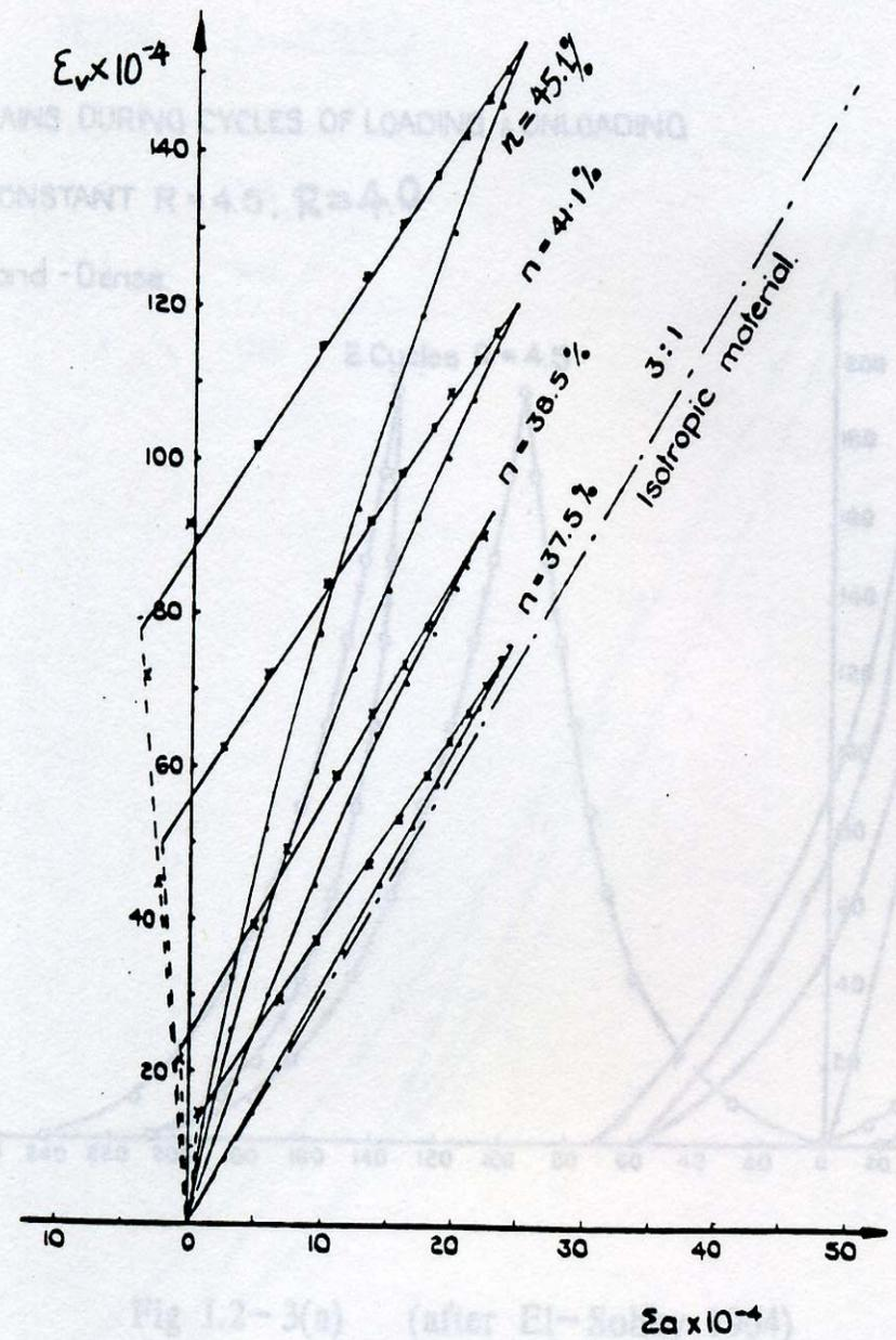
Fig I.2-1 Axial strain and volumetric strain during cyclic isotropic loading (after El-Sohby 1964)
