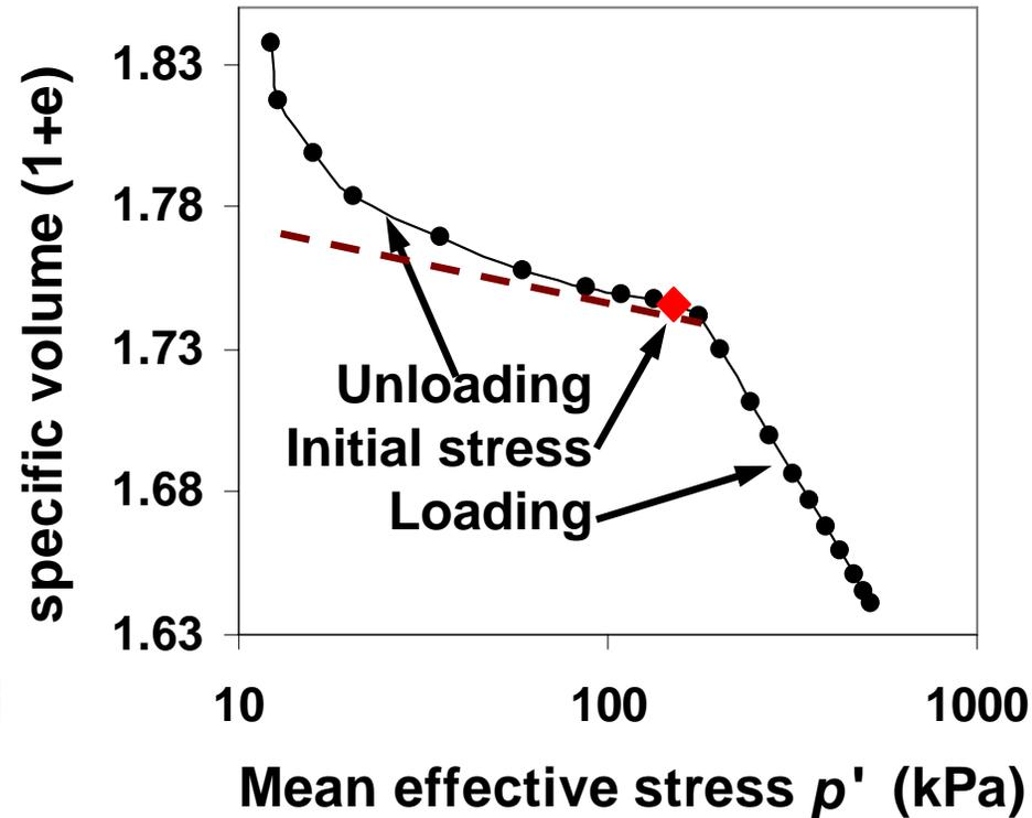
The behaviour of Beaucaire clay under isotropic loading and unloading tests (Costanzo et al, 2006)
