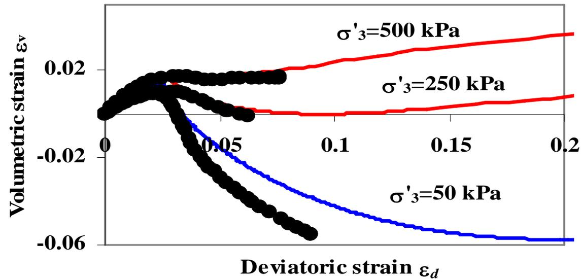
A special feature, observed in tests on most natural soft clays, Test  $\sigma'_3=50$  kPa During softening, compressive volumetric deformation seen
