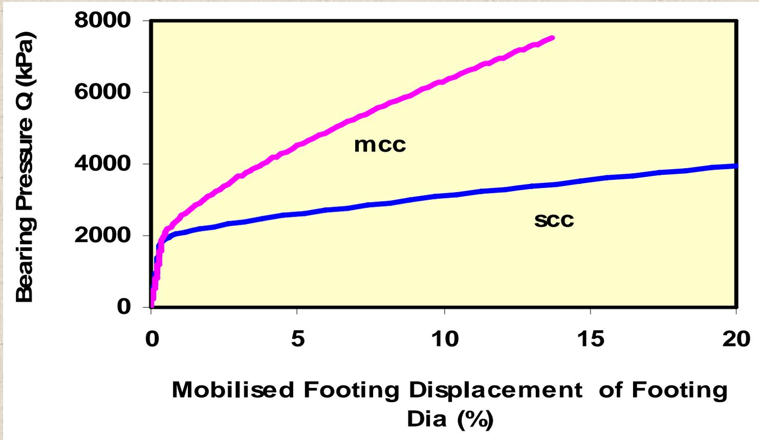
**Load-displacement response of rigid footing
