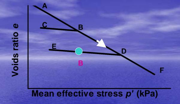
Soil behaviour for reloading  $C \rightarrow B$ , elastic When stress goes beyond B, the current stress the maximum stress the soil ever experienced
