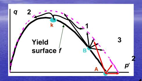
All the loading, on yield surface f, resulting the same change in the yield surface  $f \rightarrow$  the same plastic volumetric strain
