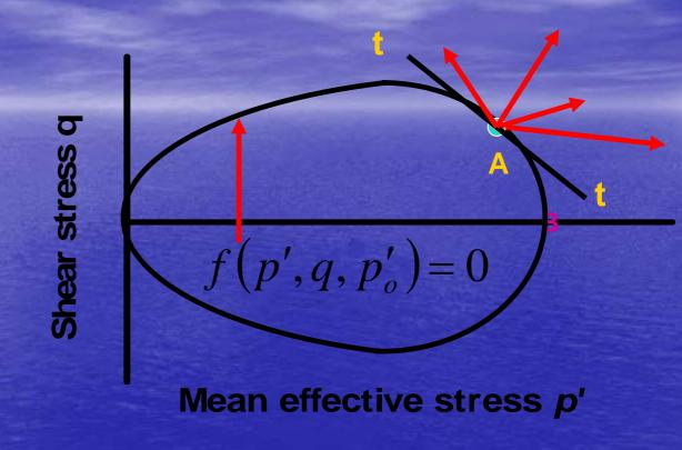
For a stress state on yield surface and with stress increment pointing outside the surface, plastic deformation occurs.
