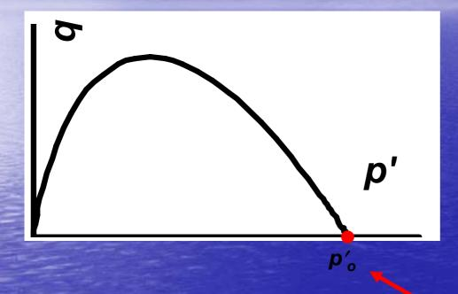
$p'_{o}$ : size of the yield surface For isotropic loading,  $\sigma'_{1} = \sigma'_{2} = \sigma'_{3}$ , then  $p' = p'_{o}$ .
