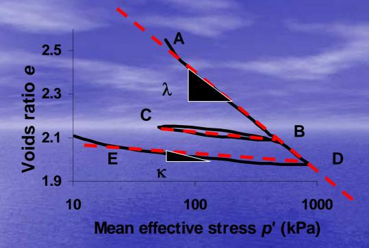
Soil behaviour for unloading BC and DE and reloading CB: also Idealized as linear.
