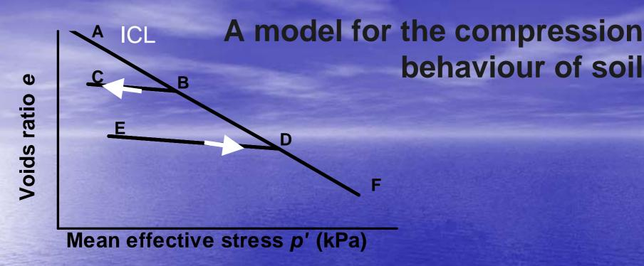
For virgin compression, current stress is maximum the soil experienced, soil behaves linearly with gradient  $\lambda$ .
