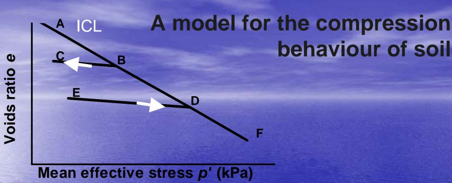
For soil behaviour with  $\kappa$ , the deformation is elastic; For soil behaviour with  $\lambda$ , the deformation is plastic.
