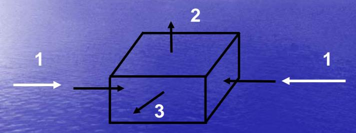
Applying stress in direction -> strain in directions 1, 2, and 3
