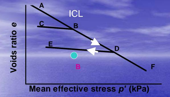
The deformation along first BD loading not elastic
