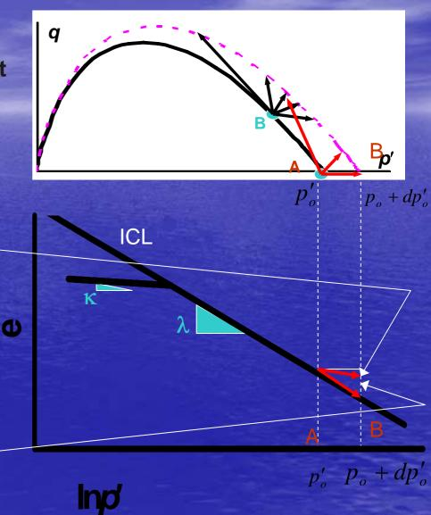
dε<sub>v</sub><sup>p</sup> obtained for yielding during isotropic compression
