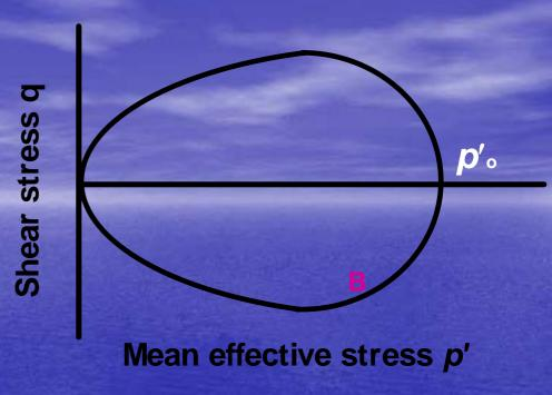
Size of the yield surface; usually p' = p' for the isotropic stress state on the surface.
