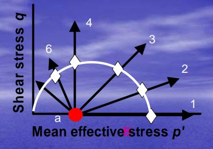
If a soil has no cohesion, e.g., non cohesive soil, tensile force cannot be applied
