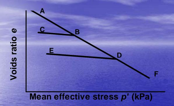
During subsequent loading, soil behaviour for unloading and reloading B→C→B, D→E→D, deformation completely recoverable elastic, described by Hook's law
